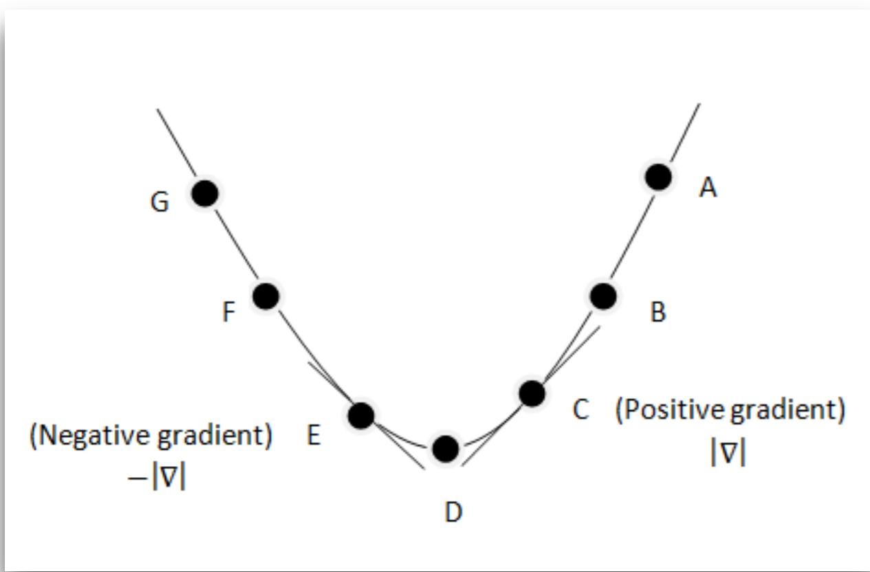
$$\begin{aligned} J &= (d - y)^2 = (d - \varphi(v))^2 = (d - \varphi(wx))^2 \\ \frac{\partial J}{\partial w_i} &= -2(d - \varphi(wx))\varphi'(wx)x_i; \\ &= -2e\varphi'(wx)x_i = -2\delta x_i \\ \alpha \delta x_i &\propto -\frac{\partial J}{\partial w_i} \end{aligned}$$
