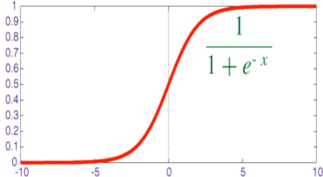
$$\begin{aligned}\varphi(v) &= \frac{1}{1 + \exp(-v)} \\ \varphi'(v) &= -1 \times \frac{-\exp(-v)}{(1 + \exp(-v))^2} = \times \frac{\exp(-v)}{(1 + \exp(-v))^2} \\ &= \frac{1}{1 + \exp(-v)} \times \frac{\exp(-v)}{1 + \exp(-v)} \\ &= \frac{1}{1 + \exp(-v)} \times \left[ 1 - \frac{1}{1 + \exp(-v)} \right] \\ &= \varphi(v)(1 - \varphi(v))\end{aligned}$$
