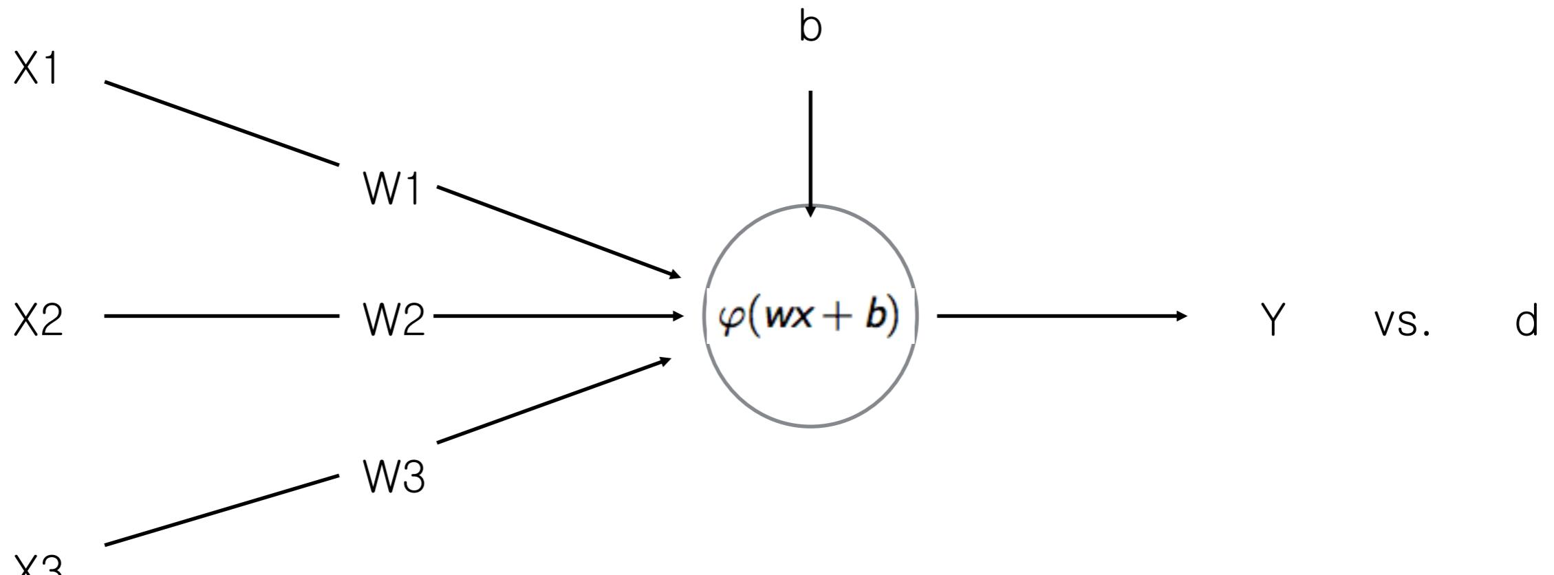
Activation function:  $\varphi(v) = v, \frac{1}{1 + \exp(-v)}, \dots$
